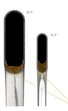
The patented stainless steel heat exchanger of the **THERMOBALANCE™** thermal unit used in the BLUEHELIX HITECH RRT (fig. A) can be compared to the most traditional and widely used steel heat exchanger (fig. B).
