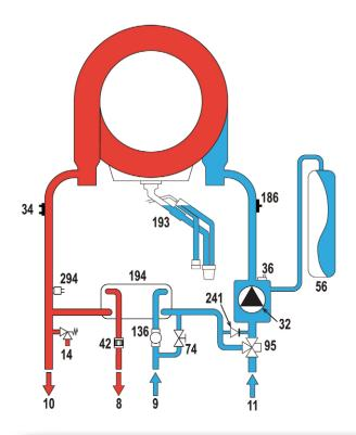
**KEY 8** DHW outlet **9** DHW inlet **10** System delivery **11** System return **14** Safety valve **32** Heating circulator **34** Heating temperature sensor **36** Automatic air vent **42** DHW temperature sensor **56** Expansion vessel **74** System filling tap **95** Diverter valve **136** Flowmeter **186** Return sensor **193** Siphon **194** DHW heat exchanger **241** Automatic bypass **294** System pressure sensor
